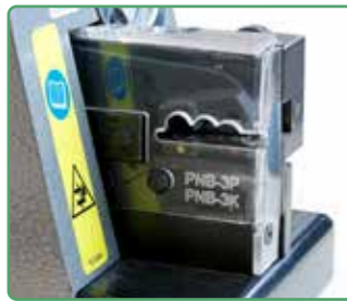
PNB-3P detail of the crimping zone.
