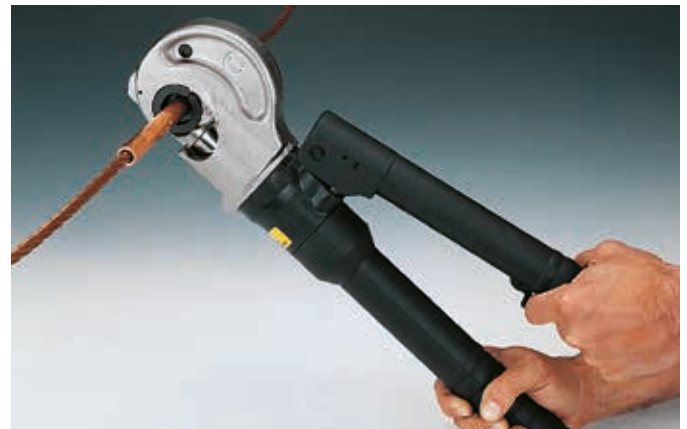
Die release system, protected from accidental operation
